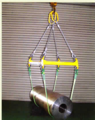
吊り天秤 (4点吊り)
